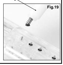
REPLACING VALVE PLUNGER ASSEMBLY (product leaks through the nozzle) IMPORTANT: Confirm that shut-offs for the position you are servicing are OFF or inclosed position (**Fig.16**, **page 6**) before replacing a Valve Plunger. Press the buttons for all positions to be serviced, to relieve pressure between the manifold and handle.
